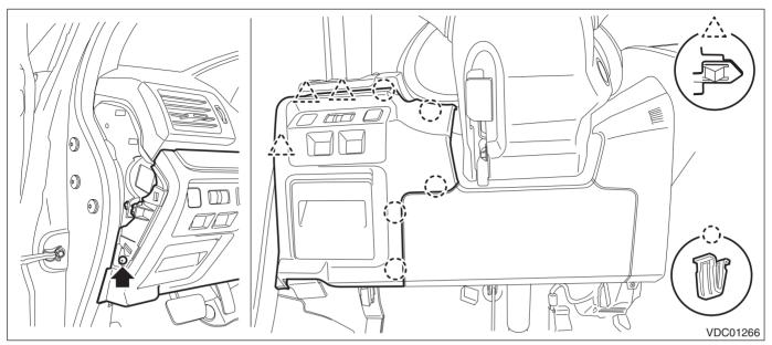
4) Remove the screws and release the claws, then detach the cover.
