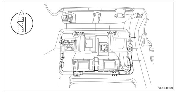
5) Release the claws and remove the VDC OFF switch.
